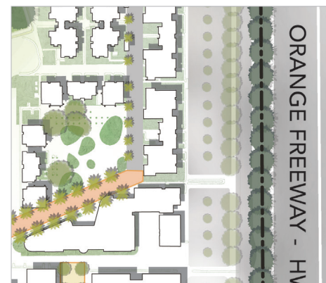
Dense landscape buffer along the highway to block noise, light pollution and air pollutions.
